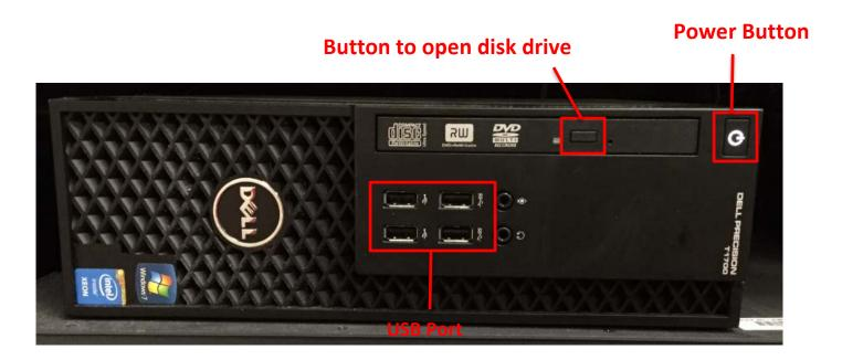
If the PC is not powered on, press the power button located on the front of the PC. The power button will light up white when turned on.
