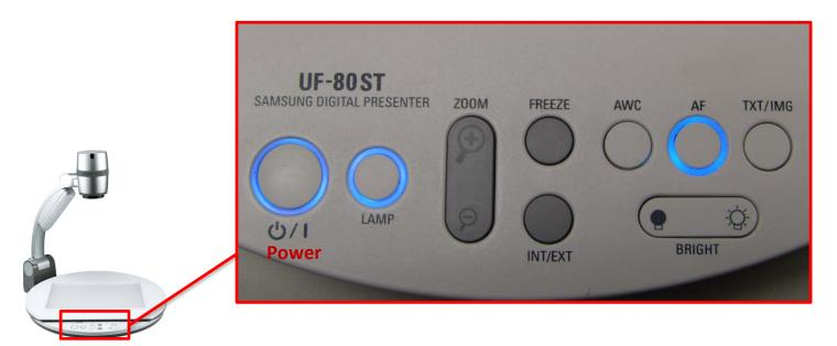
Place object you wish to project onto the base of the document camera. If you need to magnify the object or zoom out, use the **Zoom button** located on the base of Doc cam.
