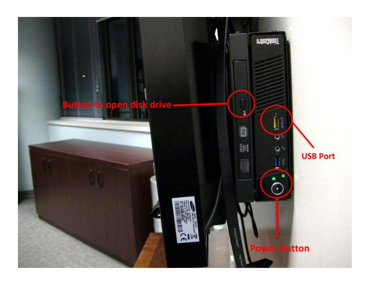
If the PC is not powered on, press the **power button** located on the front of the PC. The power button will light up green when turned on.
