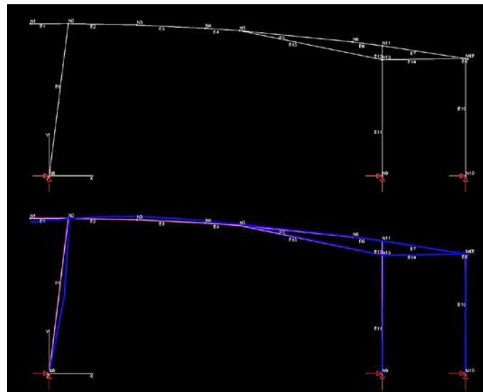
Figure 4: Top: An image of the structural analysis model (Software: MASTAN2); Bottom: the same model showing how the roof plank acts as a spring by bending under different load cases. Here, a case of upward bending the roof subjected to wind loads. [note: more on that subject in part 4 c]
