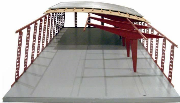
Figure 2: Partial model of a classroom building (internal partitions are omitted) with “peeled away” to reveal the roof’s different layers. (Model at Museum of Modern Art, New York).
