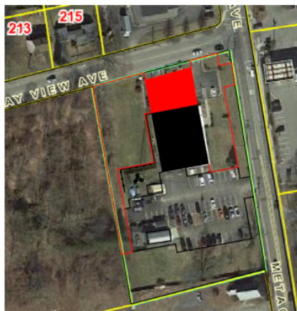
ADDITION MASSING - OPTION 2 - BAYVIEW EXTENSION - New rear and front drive and parking/ connection - New structure attached to north side of existing (adjacent to Bayview Avenue) - Public parking moved to front of building (adjacent Metacomb Avenue)
