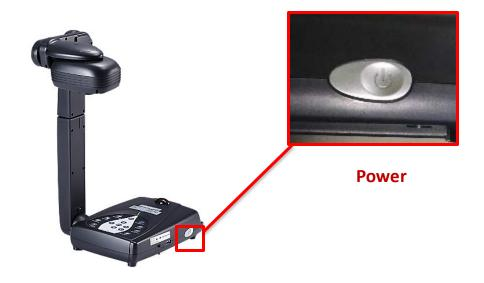
Place object you wish to project under the camera head of the document camera. If you need to magnify the object or zoom out, use the **Zoom button** located on the base of Doc cam.
