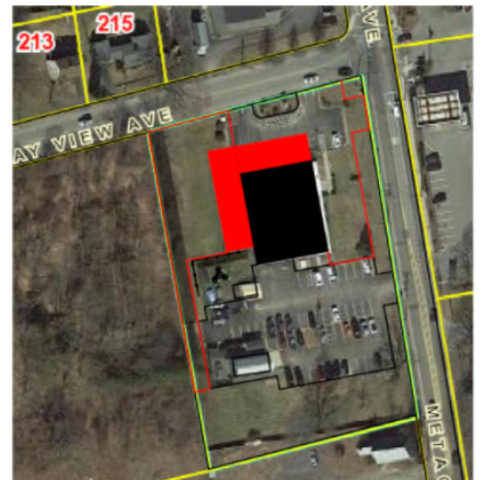
ADDITION MASSING - OPTION 3 - NORTHWEST 'L' ADDITION - New rear drive/public parking lot extension/ connection - New structure attached to back and side (west and north side) of existing - Rearranged public parking and additional squad parking
