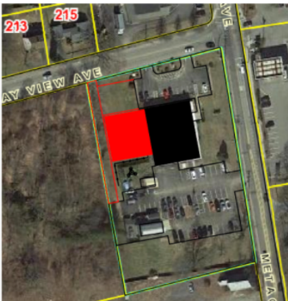
ADDITION MASSING - OPTION 1 - REAR EXTENSION - New rear drive/public parking lot extension/ connection - New structure attached to back (west side) of existing
